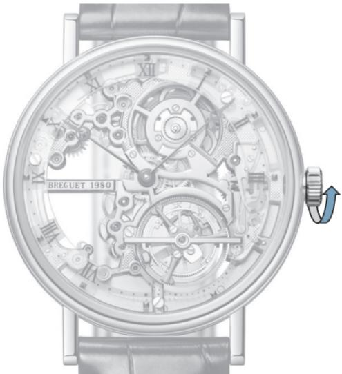
Crown in position **X1**. This position enables the movement to be wound by hand when the watch has stopped. Before performing any other operation, wind it by turning the crown upwards
