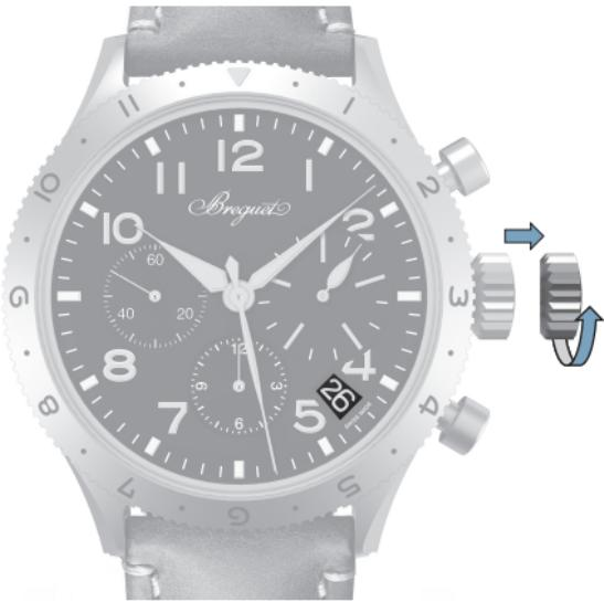
Pull the crown into position **X2**. Turn the crown upwards until the exact date appears in the aperture. Then push the crown into position **X1**.
