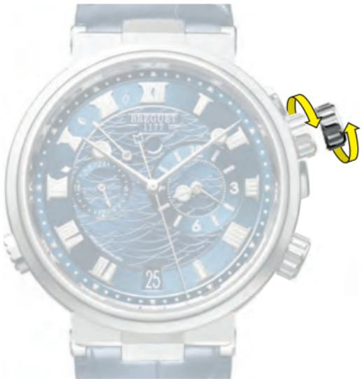
Unscrew crown **X** by turning it downwards (◐) until it moves into position **X2**. This position is used to manually wind the watch and the alarm bell. Wind the crown upwards approximately 55 turns (◑). Then apply pressure on crown **X** and screw it back into position **X1** by turning it upwards (◐). The wearer's movements then automatically wind the watch and the alarm bell. When unworn, following a complete winding, the watch will stop after about 45 hours.
