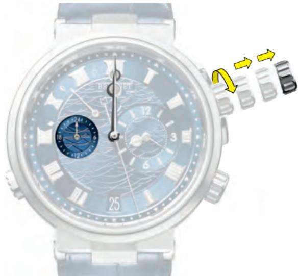
Push crown **X** back into position **X2**, then pull it into position **X3** and make the local time zone hours hand **H12** jump from hour to hour by turning the crown upwards (⌚) until the date displayed in aperture **D** changes.
