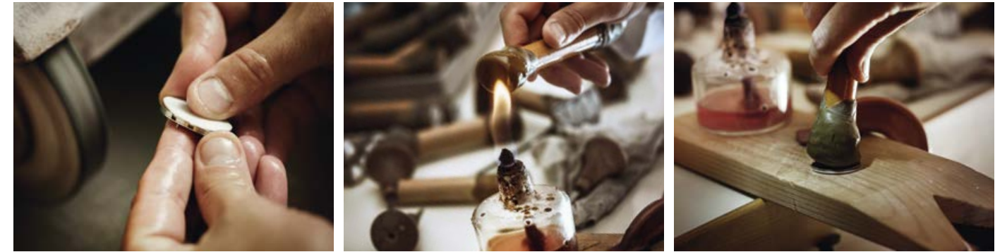
♦ Once the dial has been cut from the shell and polished, it is attached to a wooden holder with a mixture of wax and pitch.
